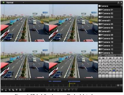
Figure 6. 27 4-ch Synchronous Playback Interface
