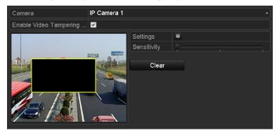
Figure 8. 12 Set Detection Area and Sensitivity of Video Tampering
