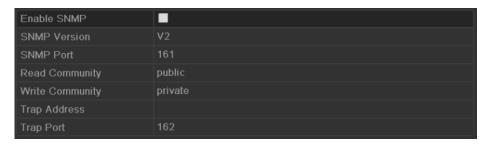
Figure 9. 14 SNMP Settings Interface
