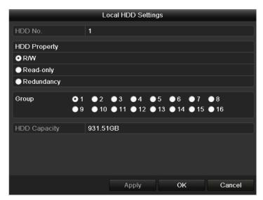
Figure 10. 13 Local HDD Settings Interface
