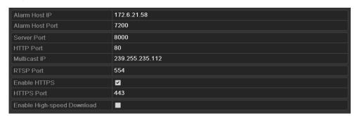
Figure 9. 22 Configure Multicast
