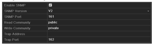
Figure 9. 15 Configure SNMP Settings
