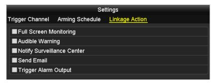
Figure 8. 5 Set Alarm Response Actions of Motion Detection
