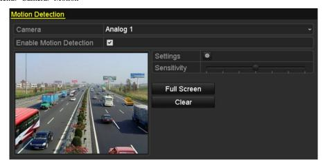
Figure 8. 1 Motion Detection Settings Interface
