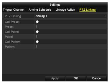
Figure 8. 10 Set PTZ Linking of Alarm Input
