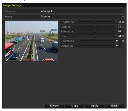
Figure 11. 5 Image Settings Interface for Analog Camera
