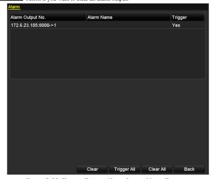
Figure 8. 22 Clear or Trigger Alarm Output Manually
