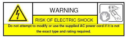
**Power Cord Requirements:** The connector that plugs into the wall outlet must be a grounding-type male plug designed for use in your region. It must have certification marks showing certification by an agency in your region. The connector that plugs into the AC receptacle on the power supply must be an IEC 320, sheet C13, female connector. See the following website for more information <a href="http://kropla.com/electric2.htm">http://kropla.com/electric2.htm</a>.
