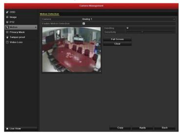
Figure 8.2 Set Detection Area and Sensitivity
