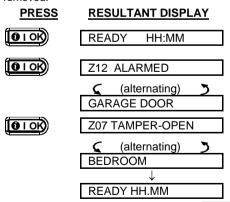
In response to additional clicking of the button, the display shows details of other events retained in open tamper (if any), or reverts to its initial state (see A above).
