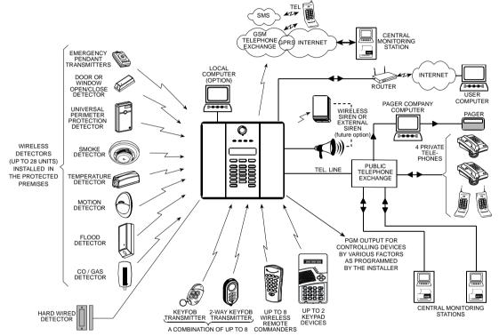
Figure 2. Typical System Configuration
