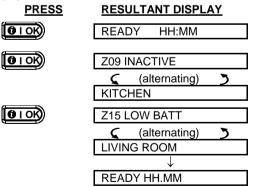
In response to further clicking of (b), the display will show details of other troubles (if any), or will revert to the initial alternating displays (see example above).
