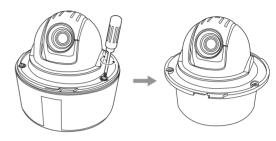
4. Connect Cables & Camera Setup Connect each camera cable to the proper terminals on the bottom of the camera (Refer to Page 13: "Camera Wiring Interface Board"). Configure the DIP switches on the bottom of the camera for communication and ID (Refer to Page 18).
